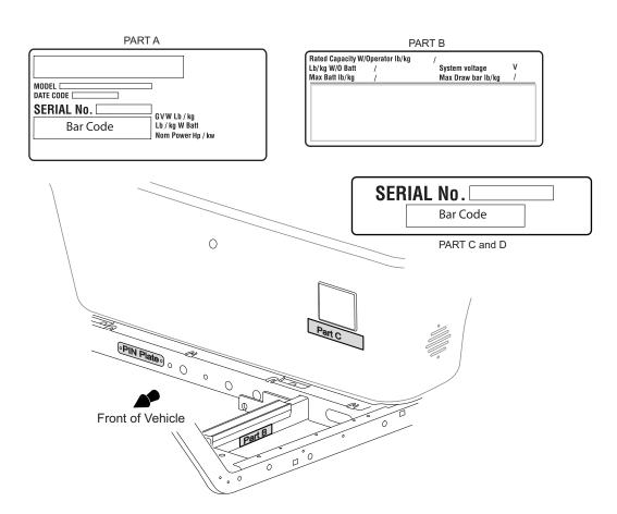
Record the vehicle identification numbers in the spaces provided below. These identification numbers are required when ordering parts from the manufacturer.
