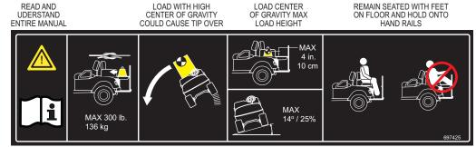
SECURE LOAD AS FAR FORWARD AS POSSIBLE MAX CARGO WEIGHT AVOID CROSSING SIDE OF STEEP HILLS MAX GRADE
