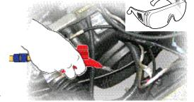
Regular maintenance of the cooling system is required to ensure an adequate supply of air to the cooling fins. Compressed air can be used for routine cooling system maintenance.
