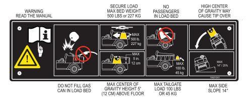
A truck bed warning label is attached to the inside front of the truck bed. Understand and comply with the warnings on this label for safe operation of the vehicle.
