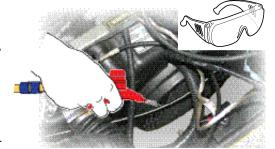
Regular maintenance of the cooling system is required to ensure an adequate supply of air to the cooling fins. Compressed air can be used for routine cooling system maintenance.
